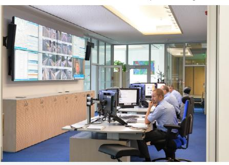
Therefore, there is a large imaging display wall made of seamless NEC LED panels. The display wall shares eight independent image sources taken from fixed or mobile traffic camera systems at intersections, highways or directly from a rescue helicopter, the current TV news on ČT 24 or GIS map sources. Picture data can be individually controlled as needed on the CUE touch panel, which includes custom-designed imaging management.
