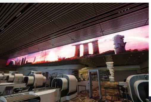
other strict RFP specifications. The new rigid Nixel technology is truly optimized for being flat with a larger diode for the highest brightness and is rear serviceable. Being able to access the displays from a high vantage point through rear service will keep traveller visibility of the displays at an absolute maximum.
