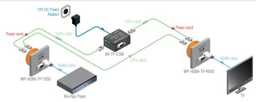
The wall and floor plates are always powered remotely in every application from the remote end device like a matrix switch or standalone transmitter or receiver. The BR-TP-COM is used as remote power source for both TX and RX side wallplates.
