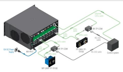
With the permanent installation of the BR-TP-COM we are able to select the active input or change EDID on the inputs of the wall and the floor plates through the control system.
